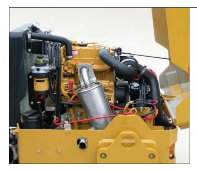
**Power.** The liquid cooled Caterpillar C1.1 engine provides a gross power of 16.1 kW (22 hp) at 2400 rpm for excellent performance with low sound levels maximizing operator comfort.
