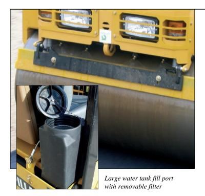
**Water Tank.** A 150 liter high-capacity polyethylene water tank is protected within the machine frame. The tank design provides extended operation and a single fill point.
