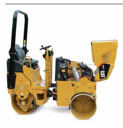
**Engine Enclosure.** Fiberglass engine enclosure pivots upward and locks open with a prop rod.
