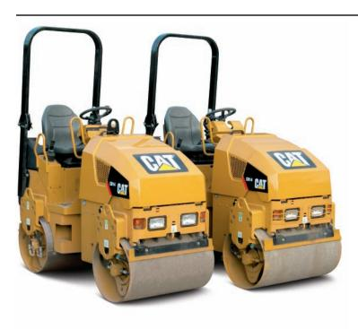
**Increased Production.** The CB14 XW is available in two versions; 900 mm wide drums and 1000 mm wide drums. These two versions enable increased mat width coverage in fewer overlapping passes.
