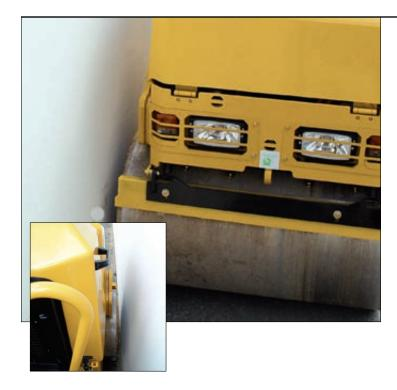
**Full flush compaction.** The front 900 mm offset driving drum allows the compactor to operate against a wall, curb or other vertical obstructions achieving complete compaction coverage.
