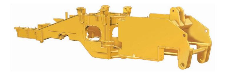
Structure Construction. Combining the use of robotic welding on up to 90 percent of the 834H with castings used in several areas contributes to increased strength by helping spread the load and reducing the number of parts. This provides highly consistent welds with deep plate penetration and excellent plate fusion. The benefit is increased durability and fatigue strength. The computer controlled machining ensures the alignment of pin bore, axle pad, cab mount and transmission/engine components.
