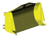
**Semi-Universal Blade.** The characteristics of the straight and universal blades are combined into the semi-universal blade (10.1 m³/13.3 yd³). It provides increased capacity with the addition of short wings which include only the dozer end bits without sacrificing spreading characteristics of straight blades.
