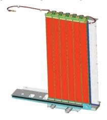
Next Generation Modular Radiator (NGMR). The parallel flow system, with six cores standard, improves cooling capabilities. Serviceability is enhanced as there is no top tank to remove. The NGMR uses copper brazed brass tubes and copper fins.
