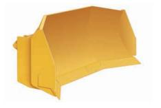
**Coal Blade.** The coal blade (22.2 m³/29 yd³) is designed for precise and productive dozing while helping to retain load control with increased capacity for lighter materials. Wing angles help retain the load while dozing. This blade is available from Cat Work Tool and Services (CWTS).
