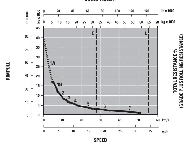
1A – 1st Gear (Converter Drive)
